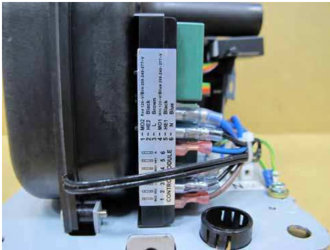
1. Remove the wires that connect motor to the timer.
