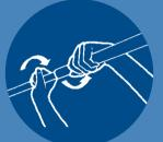
**3** further extend the rod to ensure a tight fit and twist to lock
