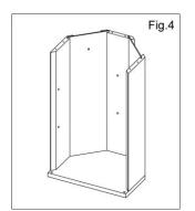
4. Locate the backing boards into the recesses on the side panels and back panel. Screw fixing holes to be positioned at the top of the cabinet. (Note- if positioned incorrectly the cabinet cannot be hung.)
