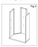
3. Secure side panel and back panel to the base using 4 fixing screws. (Screws mounted from underside of base. To improve strength place small amount of glue on underside of side panel before securing into position.)
