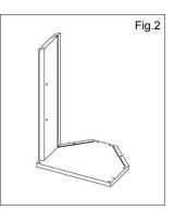
2. Secure side panel to base panel using two fixing screws. (Screws mounted from underside of base. To improve strength place small amount of glue on underside of side panel before securing into position.)
