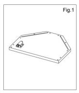
1. Mount the magnetic door catch to the top panel using the magnetic catch screws and ensure the magnetic door plate is fitted to the mirror door using the magnetic plate screw provided. The door catch must be fitted to opposite side of door hinge.
