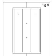
9. Hold the cabinet against the wall in its desired location and check that it is straight and level. Open the door(s) and mark the wall using the holes in the back of the cabinet as a guide. Drill 40mm deep holes in marked positions using a 6mm masonry drill and insert wall plugs. Align the holes in the back of the cabinet with the wall plugs. Insert the screws through the washers and holes in the back of the cabinet and screw in position.
