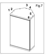
7. Place top panel onto cabinet carcase ensuring all screw holes, recesses and pivot pin bush are accurately aligned. Secure the top panel to the side panels and back panel. (Six fixing screws required.) To improve strength place small amount of glue on underside of side panel before securing into position.)
