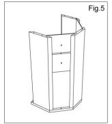
5. Slide the two strengthening batons into the channels at the rear of the cabinet with the pilot holes facing towards the top of the cabinet. Not to be secured into top panel at this stage.
