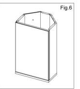
6. Place one of the door pivot pins into hole recess situated on the base panel. (The pivot pin bush needs to be located in the recess before inserting the pivot pin) Locate mirrored door onto pivot pin and place second pivot pin into the top of the door before securing the top panel.
