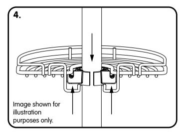
**4.** Align the 'D' shape wire profile of the basket with the 'D' shape recess in the Securing Clip and press the two components together until they click into place.
