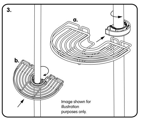
**3.** Place the basket over the Securing Clip. It may be necessary to rotate the Securing Clip through 90 degrees to allow the clip to pass through the back of the wire basket.
