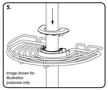
**5.** Finally, align the Cover Plate with the Securing Clip and press together to finish the assembly.
