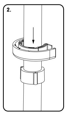
**2.** Attach the Securing Clip to the riser rail and slide it over the Collet until it is tightly fixed in the desired position on the rail.
