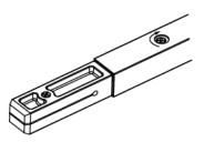
2. Assemble the second rod onto the straight joint making sure that the tube ends are pushed tightly together, align the hole with the grub screw and again clamp tightly in position (see Fig. 2).
