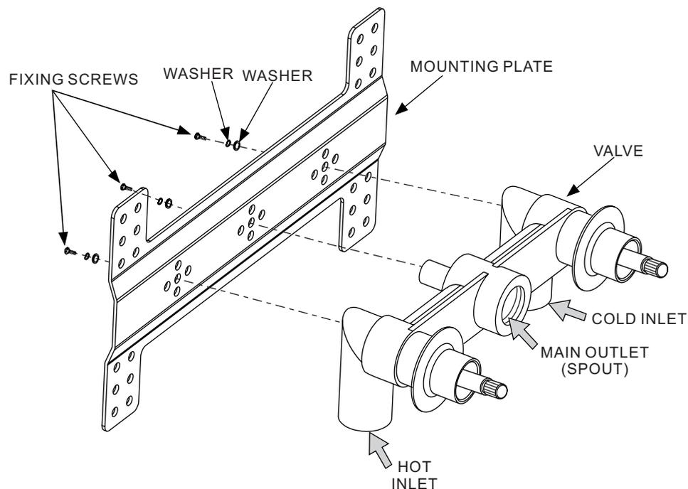
FIG. 1 INSTALLATION OF SPOUT
