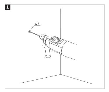
Measure area where accessory will be installed. Use drill to create hole.
