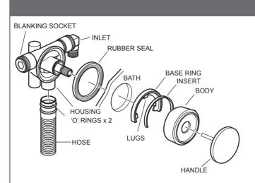
Prepare the assembly by pushing the 'O' ring onto the nut. Push the rubber seal onto the housing, and hold the unit in position from the outside of the bath. From the inside of the bath place the base ring over the bath hole, **if the hole is to small, snap off one of the lugs with a pair of long nose pliers**. Slide the insert and body into the base ring and screw on the nut, finally screw on the cover.
