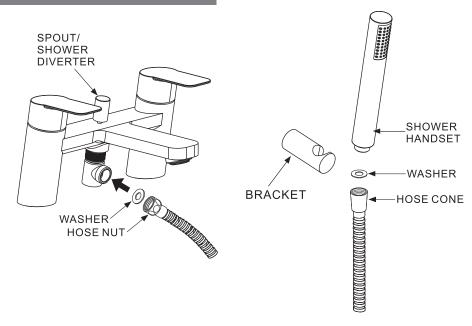
Insert a washer into the cone end of the hose and screw to the handset.
