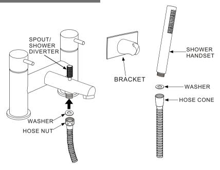
Insert a washer into the cone end of the hose and screw to the handset.
