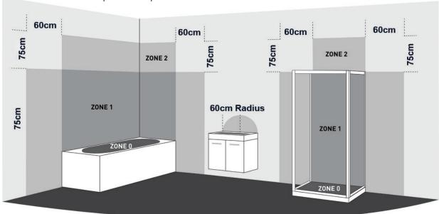
This product is IP44 rated and is suitable for installation within zone 2 above, and complies with the following safety standards: EN 60598-2-1:1989, EN 60598-1:2015, EN 62493:2015
