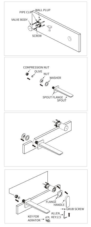
First shut off your water heating system, then with your mains Stop cock closed, open the lowest cold and hot taps in the house and allow to run until the cold storage tank and pipes are empty (the hot storage cylinder always remains full). Fitting isolating valve to inlet feeds is recommended for ease of maintenance.
