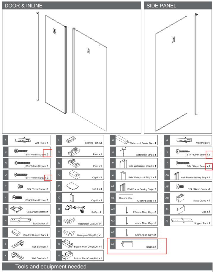
Drill, 6mm Masonry drill bit, 3.2mm General drill bit, Philips screwdriver, Spirit level, Pencil, Scissors, Knife, Silicone sealant.
