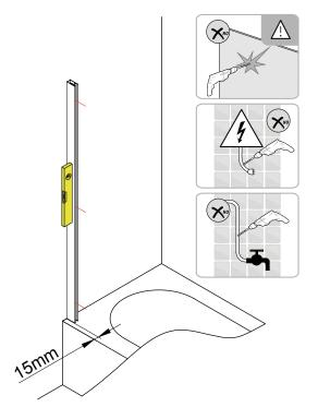
Place wall channel in position on the bath (15mm in from the edge of the bath), use a spirit level to ensure that it is vertical, and mark all 3 fixing holes on the wall.
