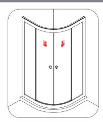
• The "up" arrow on the sliding door should be to the top, and be on the outside of the enclosure.
