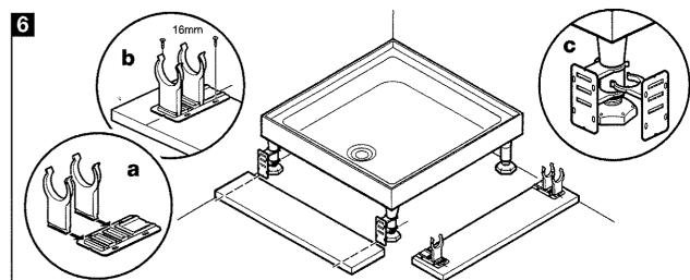
(a) Separate and assemble the panel brackets. Push fit the panel brackets onto the legs, align panel/s up with the brackets and mark the centre line of the brackets onto the back of the panel/s.
