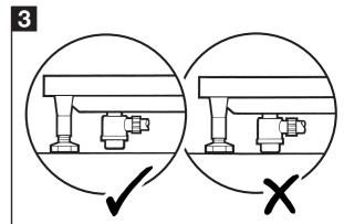
Place the tray in position and fit waste pipe. Make sure pipe work is clear of floor when standing in the tray. If necessary cut a hole in the floor to provide adequate clearance.
