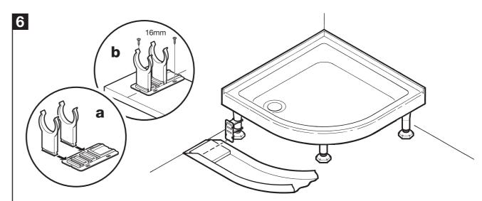
(a) Separate and assemble the panel brackets. Push fit the panel brackets onto the legs, align panel up with the brackets and mark the centre line of the brackets onto the back of the panel.
