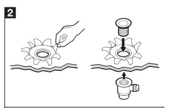
Peel back protective film from waste hole inside the tray and fit waste outlet. Fit the waste and trap as per the manufacturers instruction. **Do not apply any sealant to the underside of the tray as this will invalidate the guarantee.**
