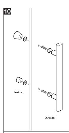
Fit the door handles (PN60510) to the door ensuring the washers fit between the glass and handle.
