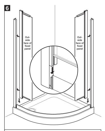
Position the fixed panels into the wall channels and slide down so that they fully slot onto the end mouldings of the bottom rail.
