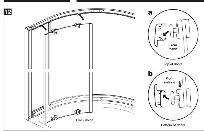
**a:** From inside the enclosure, position the top wheels into the top rail. **b:** From outside the enclosure with the door closed, push down the 'plungers' on both bottom wheels, position into the bottom rail and release. Repeat with other door.
