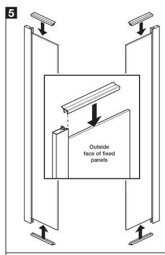
Push fit the 'flipper seals' onto the top and bottom edges of both fixed panels - flush against the metal profile. Ensure the flipper seal 'flaps' are on the inside of the fixed panels.
