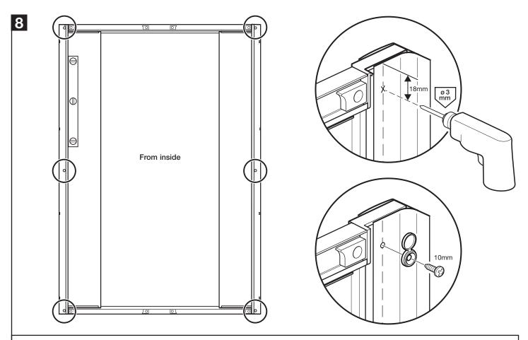
Check the door frame is vertical and is centrally positioned between the wall channels.
