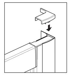
Push fit the top caps (PN50493/50494) onto the wall channels.
