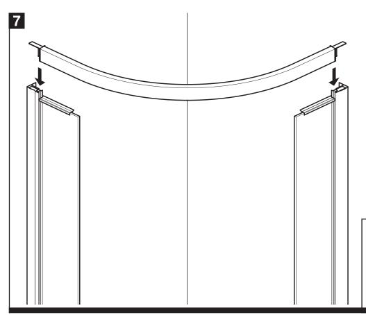
Position the top rail onto the top of the fixed panels/wall channels.
