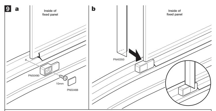
**a:** Attach 2 x glass clamps to each of the horizontal rails (at edge of glass) using 10mm screws, **tighten by hand only - do not overtighten.** Push fit glass clamp covers.
