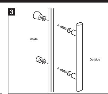
Fit the door handles (PN60510) to the door ensuring the washers fit between the glass and handle. A chrome finish handle is supplied for all frame finish options.
