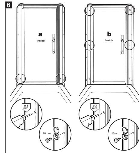
Check door is centrally positioned, perfectly vertical and square in the frame.
