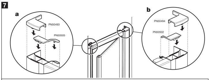
Push-fit the top caps onto the wall channels.
