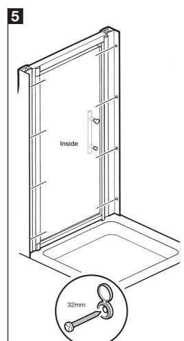
Place door in position on the tray, fix wall channels to the walls (in all 8 positions shown) using 32mm screws and screw caps.
