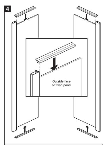
Push fit the 'short flipper seals' onto the top and bottom edges of the fixed panels - flush against the metal profile. Ensure the flipper seal 'flaps' are on the inside of the fixed panels.
