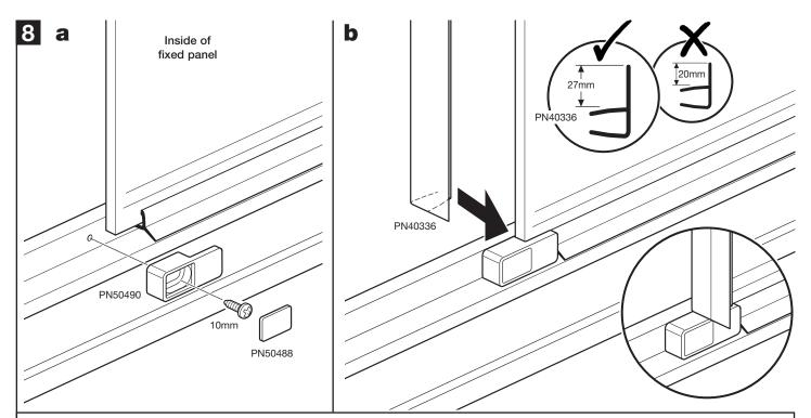
a: Attach glass clamps to each horizontal rail (at edge of glass) using 10mm screws, tighten by hand only - do not overtighten. Push fit glass clamp covers.
