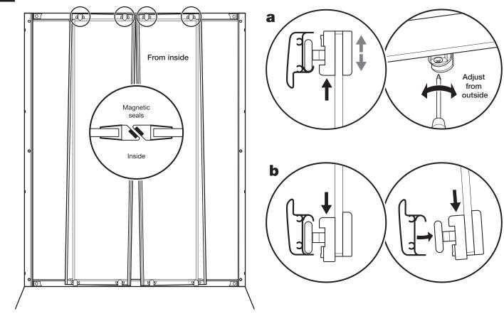
**Door adjustment:** The wheels at the top of the doors may need adjusting so that the doors slide freely and the magnetic seals meet evenly when the doors are closed.
