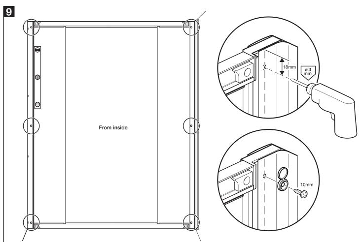
Check the door frame is vertical and is centrally positioned between the corner post and wall channel.
