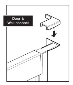
Push fit the top caps onto the wall channels and corner post as shown.
