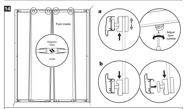
**Door adjustment:** The wheels at the top of the doors may need adjusting so that the doors slide freely and the magnetic seals meet evenly when the doors are closed.
