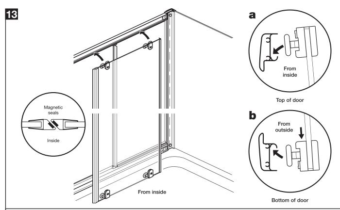
**a:** From inside the enclosure hang both doors, position the top wheels into the top rail. **b:** From outside the enclosure with the doors closed, push down the 'plungers' on both bottom wheels, position into the bottom rail and release.
