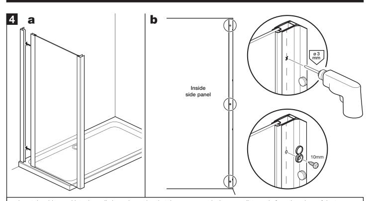
**a:** Insert the side panel into the wall channel ensuring that the corner post is the same distance in from the edges of the tray as the wall channels.
