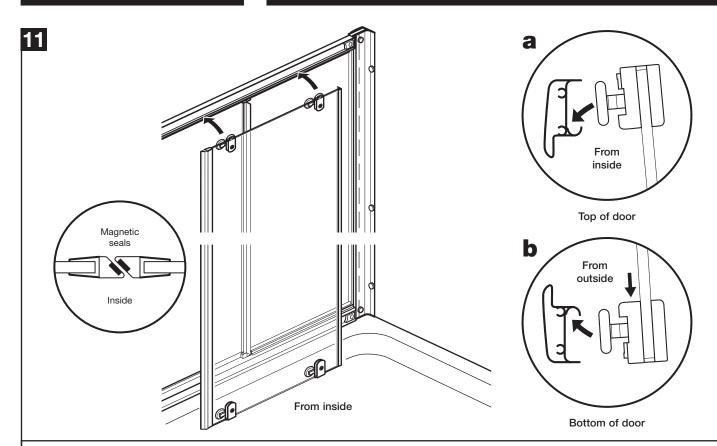
**a:** From inside the enclosure hang both doors, position the top wheels into the top rail. **b:** From outside the enclosure with the doors closed, push down the 'plungers' on both bottom wheels, position into the bottom rail and release.
