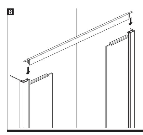
Position the top rail onto the top of the 'fixed panels'.
