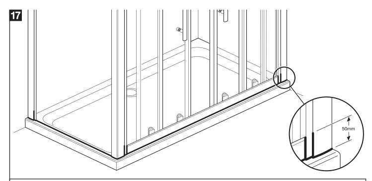
From the outside only, apply sealant to the bottom of the enclosure and 50mm up the wall channels and vertical joints as shown.
