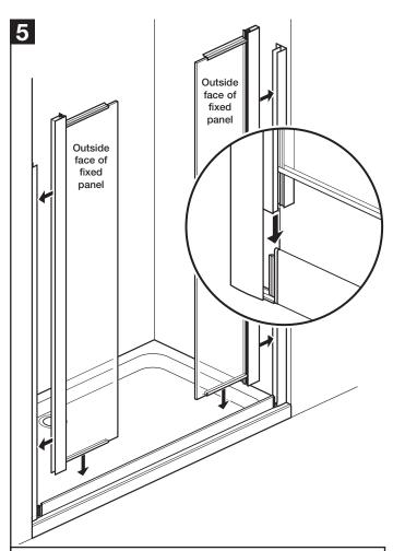
Position the fixed panels into the wall channels and slide down so they fully slot onto the end mouldings of the bottom rail.
