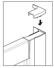
Push fit the top caps (PN50493/50494) onto the wall channels as shown
