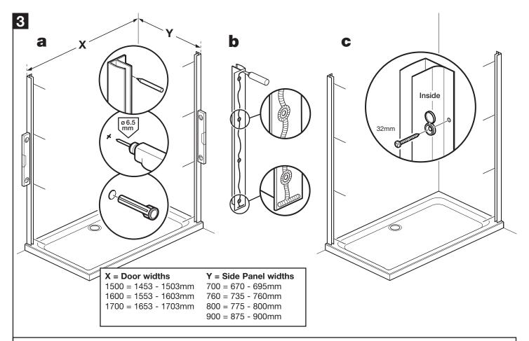
**a:** Place the wall channels on the tray ensuring they are vertical and an equal distance back from the front of the tray. Place masking tape against the wall before marking drill hole positions, this will help prevent the drill bit slipping. Drill 6.5mm holes, 30mm deep and insert the wall plugs.
