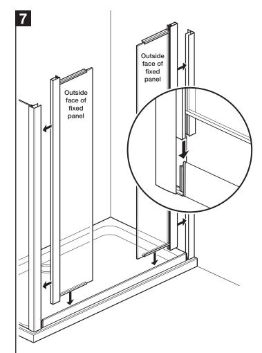
Position the fixed panels into the corner post and wall channel and slide down so they fully slot onto the end mouldings of the bottom rail.
