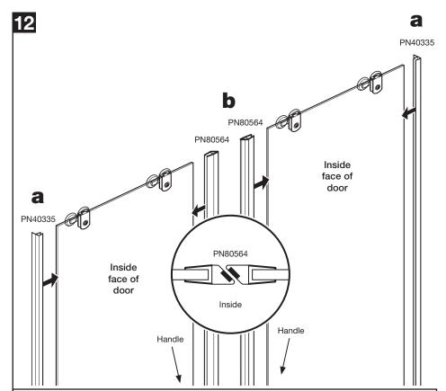
**a:** Select vertical seals (PN40335) with the 20mm 'flipper' and fit onto the back edge of the doors. **Ensure the flipper seal 'flaps' are on the outside of the doors.**
