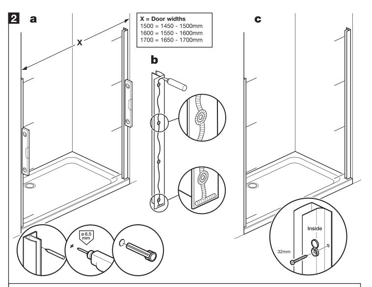
**a:** Place the wall channels on the tray ensuring they are vertical and an equal distance back from the front of the tray. Place masking tape against the wall before marking drill hole positions, this will help prevent the drill bit slipping. Drill 6.5mm holes, 30mm deep and insert the wall plugs.
