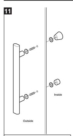
Fit the door handles (PN60510) to the doors ensuring the washers fit between the glass and handle.
