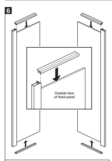
Push fit the 'short flipper seals' onto the top and bottom edges of the fixed panels - flush against the metal profile. Ensure the flipper seal 'flaps' are on the inside of the fixed panels.
