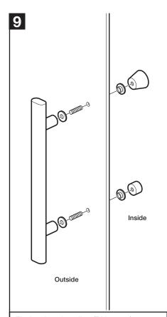
Fit the door handles (PN60510) to the doors ensuring the washers fit between the glass and handle.
