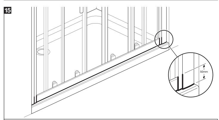
From the outside only, apply sealant to the bottom of the enclosure and 50mm up the wall channels and vertical joints as shown.
