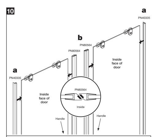
**a:** Select vertical seals (PN40335) with the 20mm 'flipper' and fit onto the back edge of the doors. **Ensure the flipper seal 'flaps' are on the outside of the doors.**
