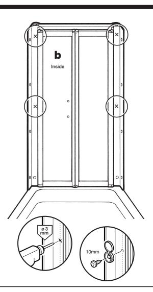
Check door is centrally positioned, perfectly vertical and square in the frame.
