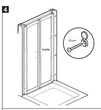
Place door in position on the tray, fix wall channels to the walls (in all 8 positions shown) using 32mm screws and screw caps.
