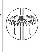
a: Partially insert grub screws into both brackets. Attach a bracket to the fixed panel, fixing through the bracket into a bracket cover using the 16mm screw, do not over tighten. Fix the remaining bracket to the wall using a 32mm screw, do not over tighten. b: Position the basket down onto the brackets and tighten the grub screws. c: Push on the bracket covers and tighten the grub screws from below.
