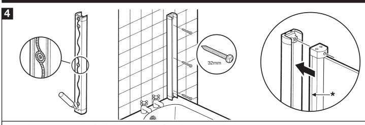
Apply silicone sealant to back of wall channel as shown. Fix wall channel to wall using the 32mm screws. Insert the bathscreen assembly into the wall channel fully tightening the top screw. The fixed panel **MUST** insert into the wall channel beyond the line marked (\*).
