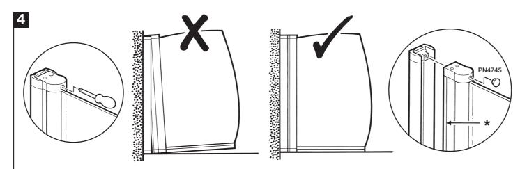
Adjust the bathscreen by tightening or loosening the screws (top and bottom) so that the bottom seal gently brushes the bath rim evenly along its length. IF THE SEAL IS TOO TIGHT ON THE BATH THE BATHSCREEN MAY LEAK.
