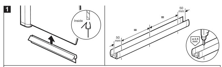
Fit the seal to the bottom of the bathscreen ensuring the seal 'flap' is on the inside of the screen, trim to length if required. Drill three holes in the wall channel (PN80277) at points shown using a 4.5mm drill bit, through the grooved centre line.
