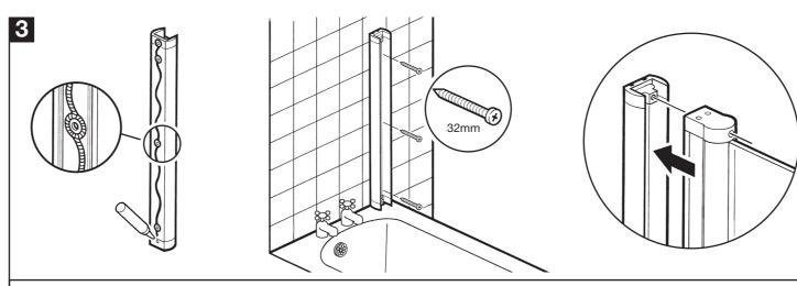
Apply silicone sealant to back of wall channel as shown.
