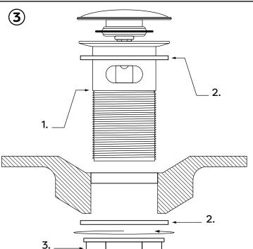
Place a 'Rubber Seal' (2) over the threaded tail of the 'Click-Clack Waste' (1). Proceed to feed the 'Click-Clack Waste' through the basin waste hole.
