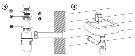
Place the 'Silicone O-ring' (A) over the threaded tail of the basin sink waste then screw the 'Top Screw Nut' (B) to the sink waste. Place the 'Silicone O-ring' (C) over the threaded tail of the 'Top Screw Nut' then slide the 'Body Tube' (D) upwards so that it reaches the sink waste and Tighten. Tighten all the 'Nuts' to ensure a tight seal. Turn on the water supply, run the tap and check all joints/connections for any leaks.
