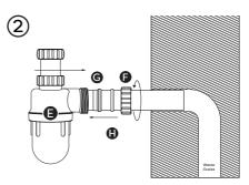
Place the 'Bottle Trap Body' (E) over the waste pipe, then fit the 'Silicone Seal' (G) and 'Plastic O-ring' (H) within the threaded tail. Screw the 'Body Nut' (F) to the 'Bottle Trap Body' ensuring a tight seal.
