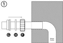
Place the 'Body Screw Nut' (F), 'Plastic O-ring' (H) and 'Silicone Seal' (G) over the waste pipe (not included) as shown in the diagram above.
