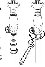
Connect the valve body to the threaded tail within the radiator and tighten the union nut using an adjustable wrench forming a water tight seal.
