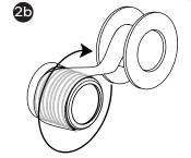
Unscrew the side union nut and threaded tail from the valve body. Wrap PTFE tape around the threaded tail to ensure a water tight seal.
