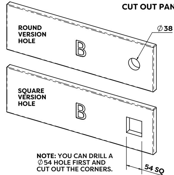
NOTE: YOU CAN DRILL A Ø 54 HOLE FIRST AND CUT OUT THE CORNERS.
