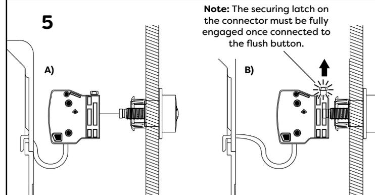
Note: The securing latch on the connector must be fully engaged once connected to the flush button.
