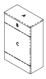
CHOOSE WHICH SIDE OF THE WC UNIT YOU WISH TO FIT THE FLUSH BUTTON IN PANEL B. CLEARANCE IS REQUIRED BEHIND THE BUTTON. IT MUST BE TO THE SIDE OF THE INTERNAL WATER TANK
