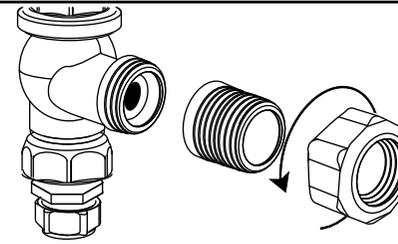
Unscrew the side union nut and threaded tail from the valve body. Wrap PTFE tape around the threaded tail to ensure a water tight seal.
