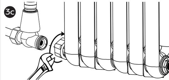
Feed the union nut through the threaded tail, then screw the threaded tail to your chosen radiator. Secure the connection using an Allen key.
