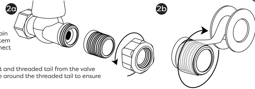
Unscrew the union nut and threaded tail from the valve body. Wrap PTFE tape around the threaded tail to ensure a water tight seal.
