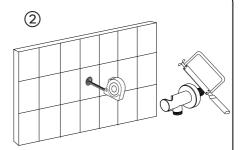
Measure the depth of the desired outlet in the wall and cut the appropriate length on the threaded tail if necessary.
