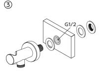
Secure the elbow holder to outlet in the wall using the o-rings and back nut provided.
