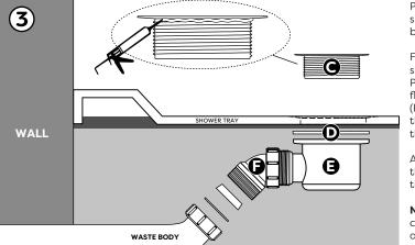
Pipe a fine bead of good quality silicone sealant around the bottom edge of the 'Flange' (C).
