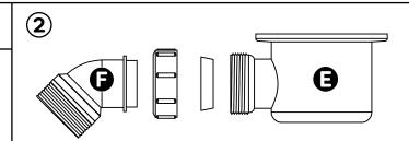
Attach the 'Trap Outlet' (F) to the 'Waste Trap' (E) and tighten.
