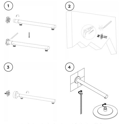
Ensure that the shower head and arm is securely fixed to the wall before use.
