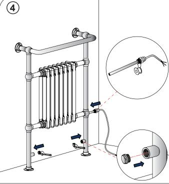
Connect to the electric supply via a fused spur. Then check for leaks. At all times follow the installation instructions supplied with the Summer Electric Heating kit. All electric work must be done by a suitably qualified person.
