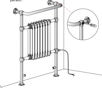
If the radiator is to be used for electric heating only ( not connected to a central heating system ), then seal the bottom inlet / outlet nipples with the blanking plugs.
