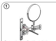
Determine the final installation position, mark the fixing hole positions in pencil.
