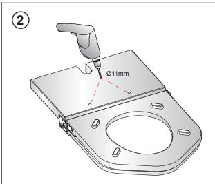
Turn the seat over, and place on a protective mat. Drill holes (recommended depth 15mm) in the marked positions using the Ø11mm drill bit.
