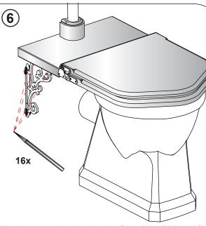
Place the ornate bracket into the fit position. Mark the fixing hole positions onto the wall and the seat by pencil.
