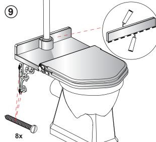
Reposition the seat against the wall, align the ornate bracket holes with the predrilled holes on the wall, fix onto the wall by tightening the screw supplied. Finally attach the back board to the wall and seat using a suitable mastic for use with wood and tiled surfaces.
