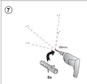
Drill holes using the Ø6mm drill bit following the marked positions, and insert the wall plugs.
