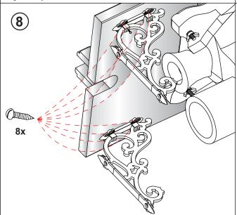
Fix the ornate bracket onto the seat with the screws supplied following the mark positions.
