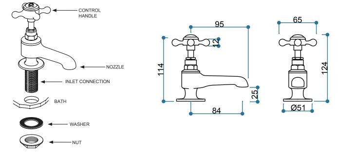
Identify the hot tap and position into the bath on the left hand, from the underside of the bath fit the rubber washer and then the nut. Making sure the tap is in the right position tighten the nut to secure the tap to the bath.
