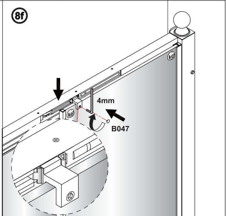
Make sure the door is closed well and there are no gaps. As indicated in the diagram between the clasps of the mechanism place the catch over the glass, and tighten to glass.
