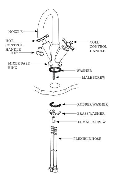
First shut off your water heating system, then with your mains stop cock closed, open the lowest cold and hot taps in the house and allow to run until the cold storage tank and pipes are empty (the hot storage cylinder always remains full). Fitting isolating value to inlet feeds is recommended for ease of maintenance.
