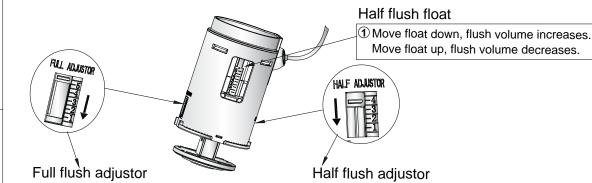
2 Move adjustor down, flush volume increases. Move float up, flush volume decreases.
