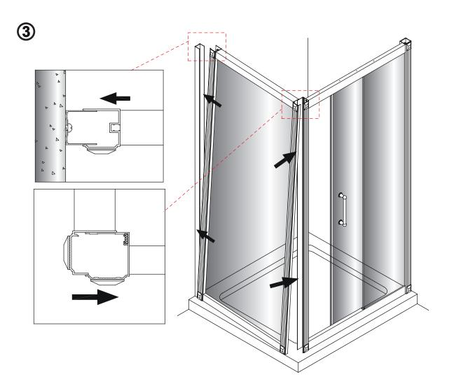
Once you have checked that the door opens and closes correctly, fix the door frame to the wall channels.
