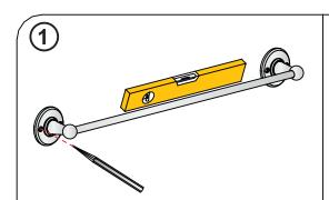
Determine the final installation position, mark the fixing hole positions in pencil.
