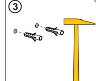
Insert the rawl plugs into the drilled holes.
