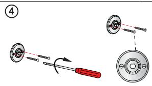
Screw in the stainless steel screws to secure the base to the wall.
