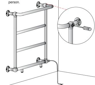
If the radiator is to be used for electric heating only ( not connected to a central heating system ), then seal the bottom inlet / outlet nipples with the blanking plugs. Fill the radiator approximately 90% with a water mixture. containing a rust inhibitor – failure to do this will lead to leaking as the radiator rusts from the inside. Filling with more than 90% liquid will lead to leaking as the water
