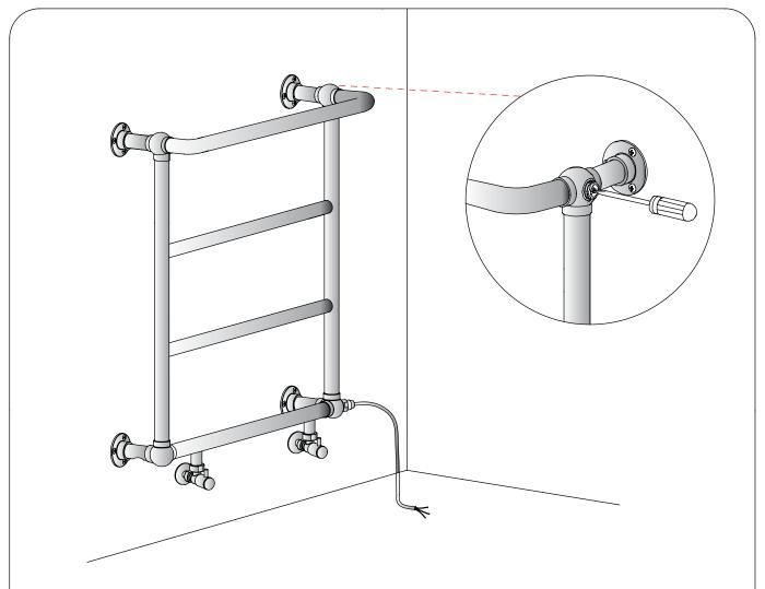
Connect to the electric supply via a fused spur. Then check for leaks. At all times follow the installation instructions supplied with the Summer Electric Heating kit. All electric work must be done by a suitably qualified person.
