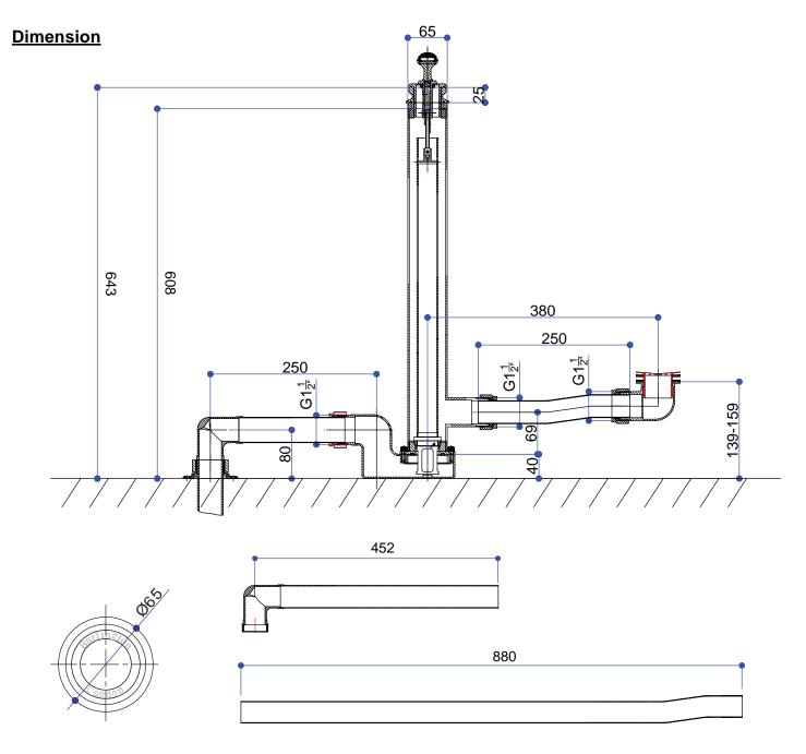
Based on the different installation condition, you may need the outlet extension, waste extension and cover plates for overflow hole included in the complete Fire Hydrant box. The cover plate kit is designed for baths with pre-drilled overflow hole.
