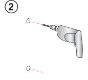
Using a 6mm drill bit, drill holes on the marked positions.
