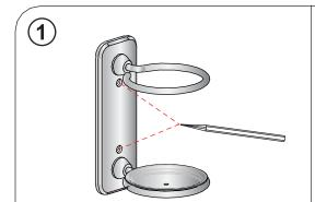
Determine the final installation position, mark the fixing hole positions in pencil.
