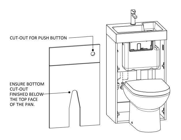
6. REFIT PANELS, CONNECTING FLUSH AND THEN SEAL WHERE REQUIRED.
