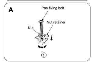
1 Unscrew the nut from the pan fixing bolt. Remove the nut retainer from the pan fixing bolt.
