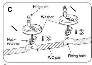
(3) Flip the nut retainer into a vertical position and insert through the pan fixing hole as shown in Figure C 3.
