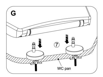
Attach the WC seat onto the hinge pins as shown in Figure G 7.
