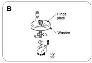
Insert the pan fixing bolt through the hinge plate and the washer.
