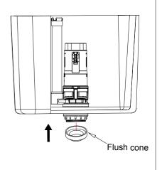
Push the flush cone over the fixing nut, ensure that it is flat, and there will be no leakage between cistern and pan.
