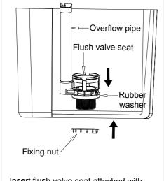
Insert flush valve seat attached with rubber washer into cistern flush hole. Then install and tighten with the fixing nut.
