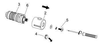
3. Assemble the cartridge(3) back to the vavle body, tighten by screwing the hex with the hex wrench, put the stop ring(6) back to the cartridge(3) and fix the handle by screwing the screw.
