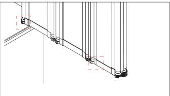
3. Remove the glue residual from the glass on both ends.
