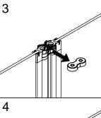
3. Disassemble the hinge.
